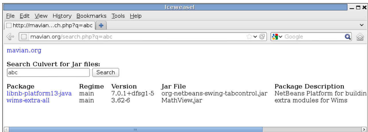
Figure 5: Culvert also offers a search mechanism. Users can search for Jars, and search results either match against Jar filenames or Debian’s package descriptions.
