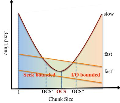
Fig. 6: The Read Time vs. the Chunk Size
