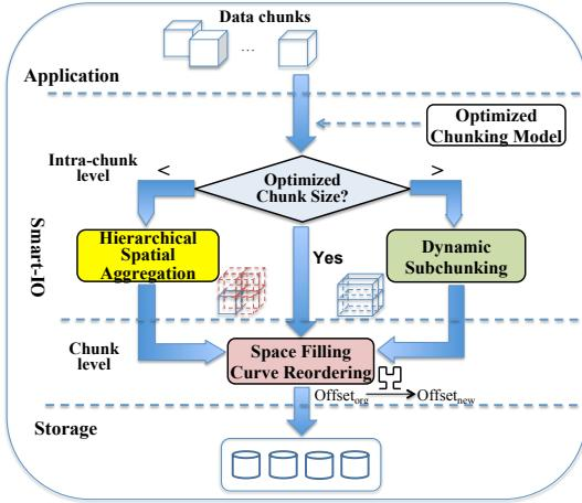
Fig. 5: Two-Level Data Organization of Smart-IO
