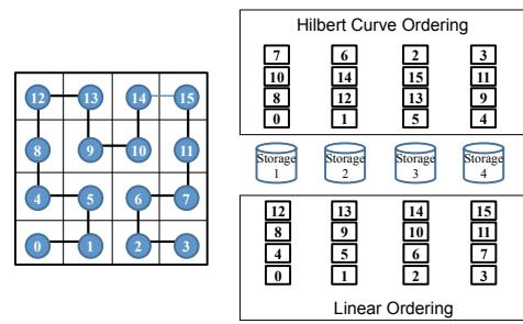
Fig. 10: Comparison of Linear Placement and Hilbert Curve Reordering of 16 Chunks on 4 Storage Nodes
