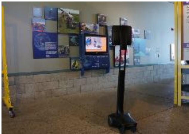
Figure 1. The Beam+ interface for the remote operators
